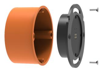
Use the screw slots top and bottom to fix the Bus Connector to the back box. You can rotate the Bus Connector within the bounds of the screw slots to ensure it is level.
