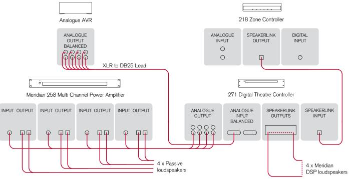
This is a 7.1 system based on a 271 in conjunction with an AVR system with balanced analogue outputs. It uses Meridian DSP loudspeakers for the front channels and the subwoofer, and passive loudspeakers for the side and rear channels; these are powered by four channels of a Meridian 258 Eight Channel Amplifier.
