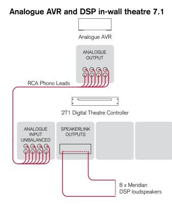
This is a 7.1 system based on a 271 in conjunction with an analogue AVR system.
