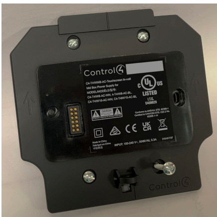
Figure 7: Secure power box to wall box
