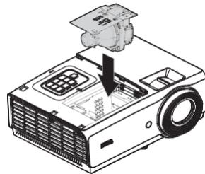
8. Tighten the screws that secure the lamp.
