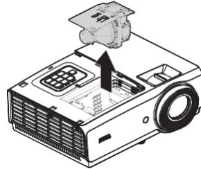
7. Insert the new lamp into the lamp compartment and make sure it fits in the projector.
