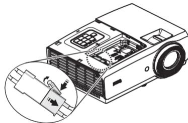
5. Loosen the two captive screws that secure the lamp.
