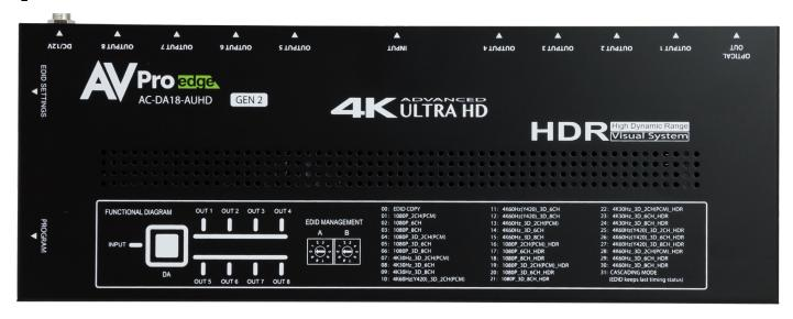
Top of the device lists the available built in EDIDs. Default out of the box the rotary dials will be set to 00: EDID COPY. This will copy the EDID from the Sync device connected to the HDMI OUTPUT #1.
