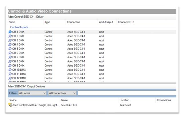
Gateway driver shows all available 512 channels. Assign channels to the Light Drivers (drag and drop).
