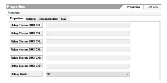
XXX Connected on CH Automatically shows the channel assigned in Connections
